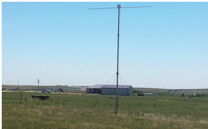
Figure 5. A temporary scientific field site hosted an ionosonde in Lusk, Wyoming. The background shows also the eclipse-watching auto traffic (to the left) lining up on the highway. Photo credit: John Swoboda (MIT Haystack Observatory).
